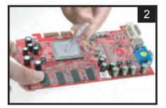
Apply an appropriate amount of thermal grease to the GPU.
