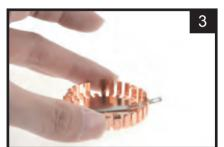
Select a suitable clip and place it onto the heatsink.
