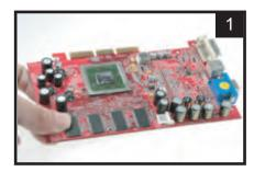
Remove the original VGA cooler
