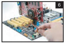
Connect the power connector to the fan header on the motherboard.
