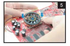
Push the push pins into the mounting holes.
